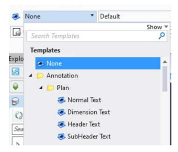
The use of the Dimension Text element template is intended for text elements in tables so that the text fits appropriately. All dimensions and table text elements should use the Dimension Text element template resulting in the same text style and level being used.
